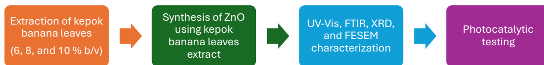
Figure 1. Schematic diagram of the synthesis process of ZnO using kepok banana leaves extract.
