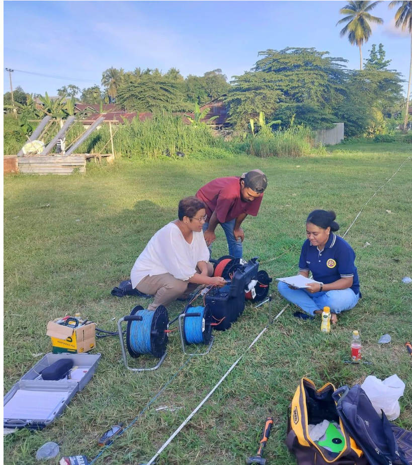
Figure 3. 1-D VES resistivity data measurement at Station I (ST-1). The AB spread ranges from 2 to 120 m, and the MN range is 1-40 m.
