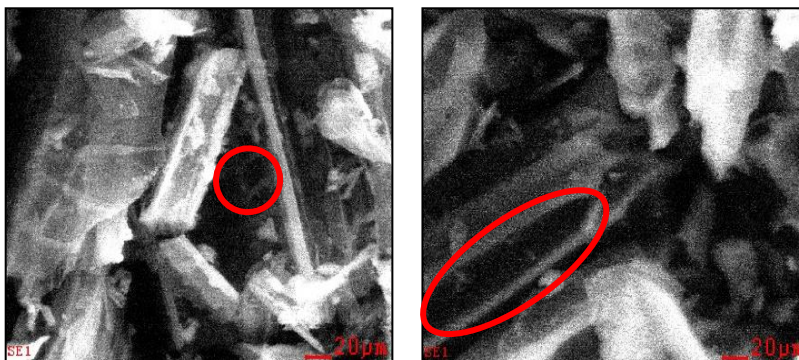
Figure 2. SEM images of (a) 60 mesh and (b) 120 mesh water chestnut 2 hours carbonization.
