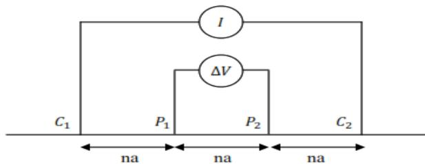
**Figure 1.** Current and potential electrodes in the Wenner configuration [16].
