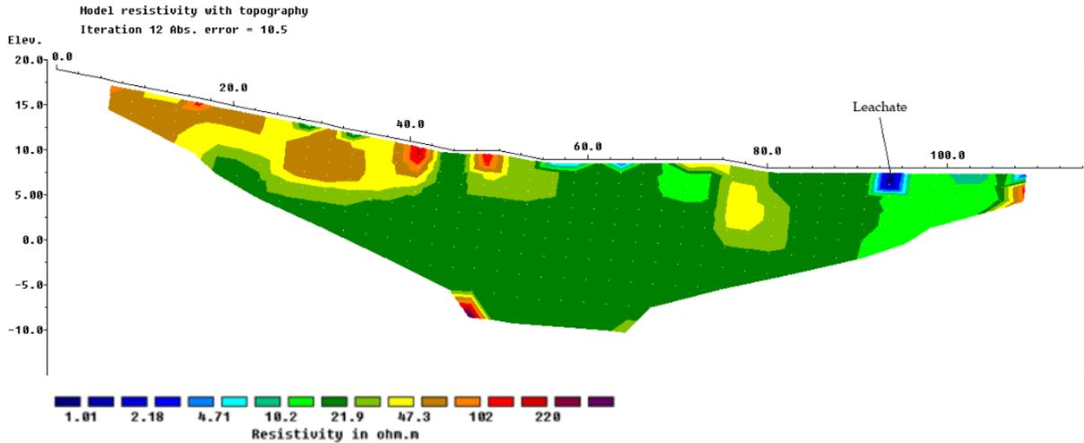
**Figure 6.** Subsurface Cross Section of Line 6
