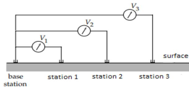
Figure 2. Fixed base configuration [14].
