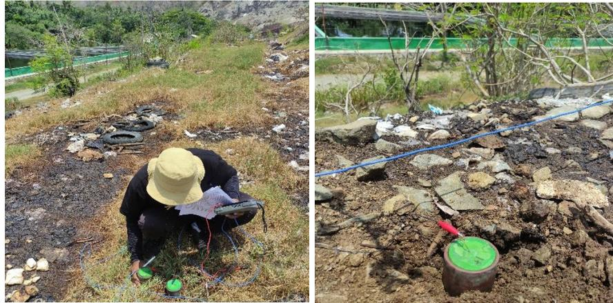
**Figure 9.** Leachate puddle conditions when taking SP measurements
