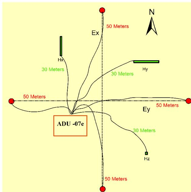
**Figure 3.** Magnetotelluric arrangement in the internal coordinate system [30].
