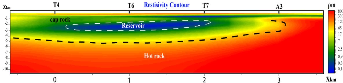
Figure 6. 2D resistivity cross section model
