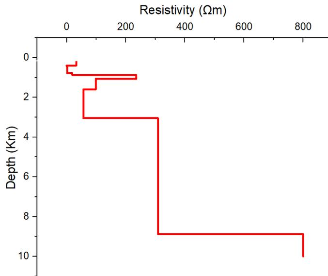
**Figure 5.** Graph of resistivity against depth in 1D at point A3
