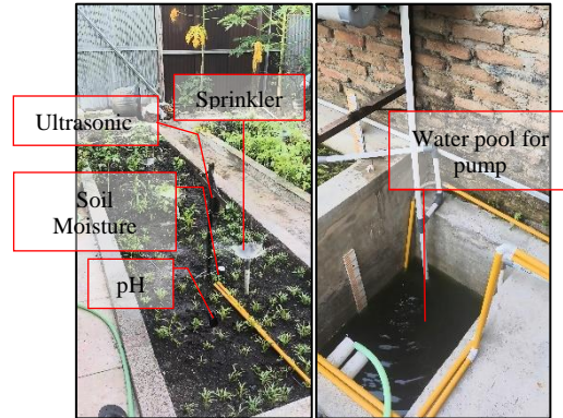
Figure 9. The condition of the land and water source pond when the watering pump is operating
