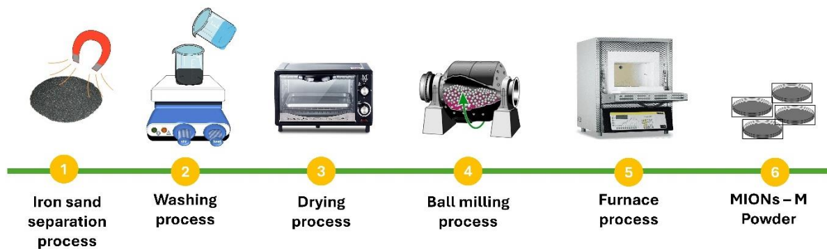
Figure 1. Illustration of mechanochemical preparation of MIONs-M Samples
