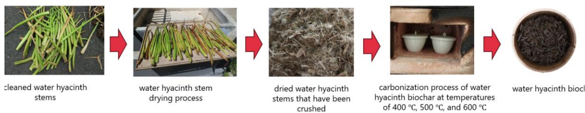
Figure 1. Synthesis procedure of water hyacinth biochar
