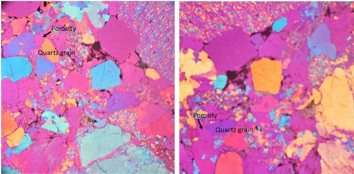
**Figure S6.** The distinction between porosity and grains can be observed using a mica comparator. In the initial observation (**Left**), porosity appears purple while the quartz grain is yellow. After rotating the sample position (**Right**), porosity retains its color, but the quartz grain shows a color change.
