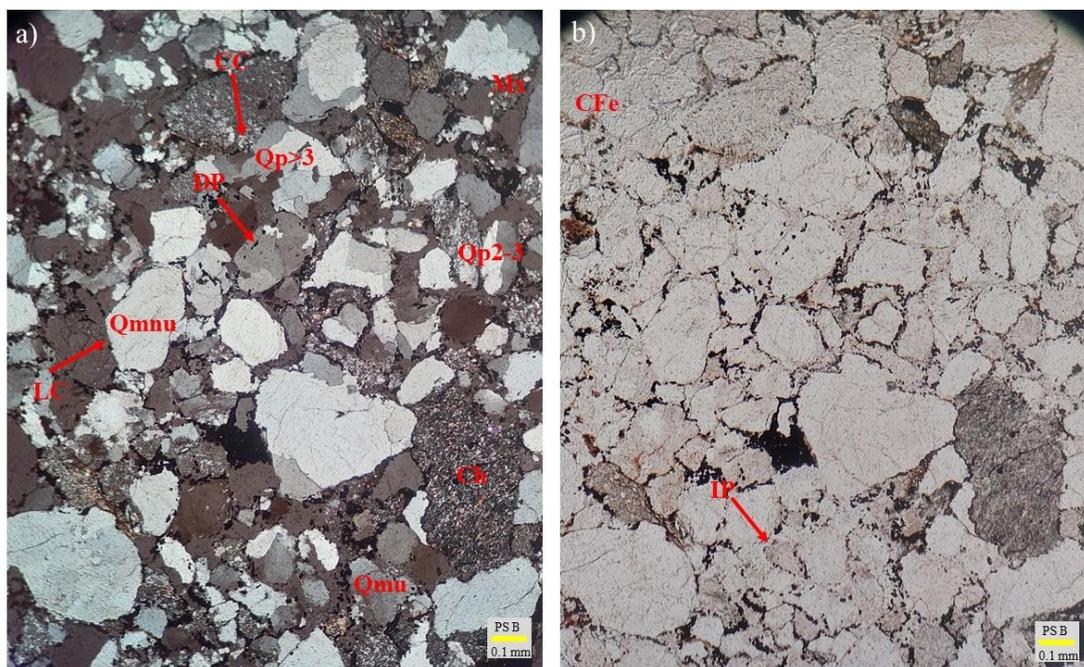
**Figure S1.** Two methods of microscopic observation: (a) cross-polarized light (XPL), (b) plane-polarized light (PPL). Grains will be more easily observed in XPL, while oxide cement is easily observed in PPL.
