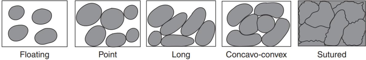
**Figure S5.** Illustrating diagram of grain contacts
