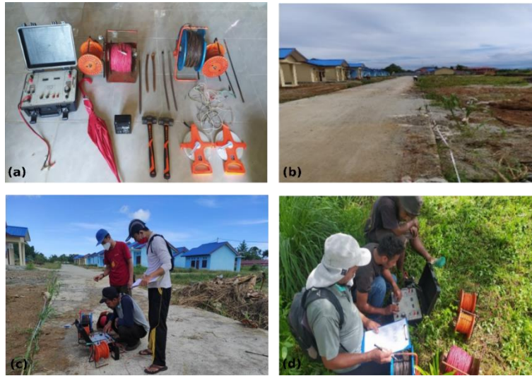
Figure 4. (a) NANIURA NRD 300 plus resistivity meter and accessories; (b) Resistivity geoelectric method measurement path at the study location; (c) Wenner configuration resistivity measurements; (d) Schlumberger configuration resistivity measurements.
