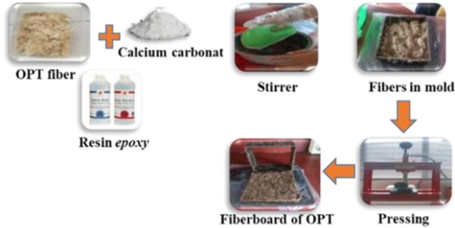
Figure 2. Stages of fiberboard fabrication
