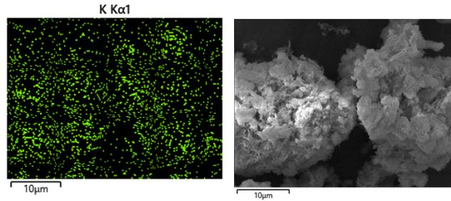
**Figure 7.** Mapping elements contained in 70:30 composition clay-carbon ceramics
