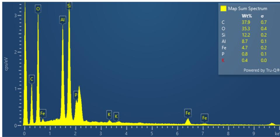
Figure 6. Elemental content in 70:30 composition clay-carbon ceramics
