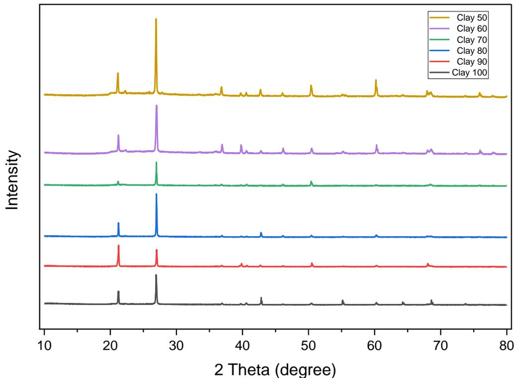
**Figure 8.** X-ray Diffraction Patterns of Clay-Carbon Ceramic Samples of each Composition
