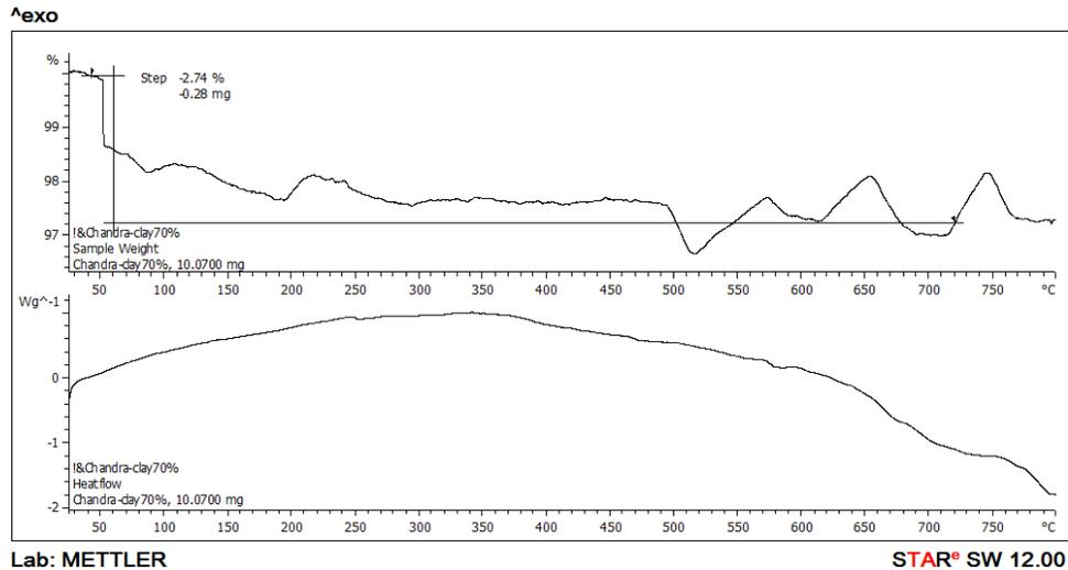
Figure 4. TGA-DTA graph of clay-carbon ceramic with 70:30 composition
