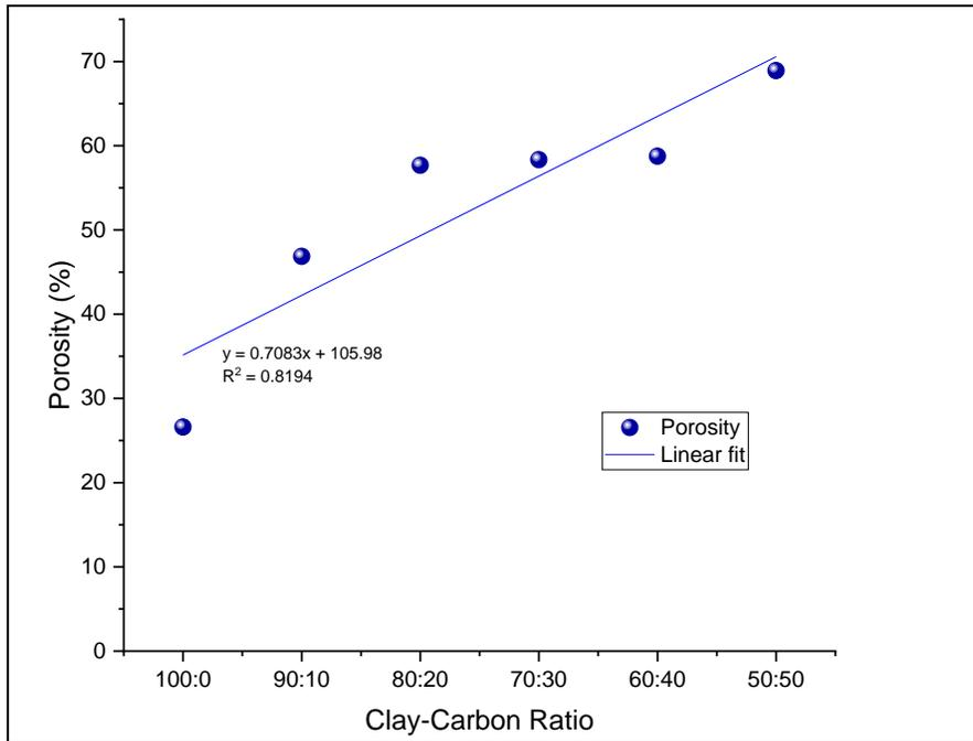
**Figure 2.** Relationship between the sample's porosity and the clay-carbon composition
