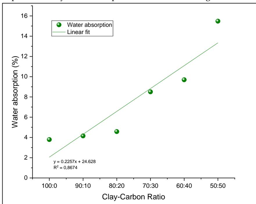
Figure 3. Relationship between the sample's water absorption and the clay-carbon composition
