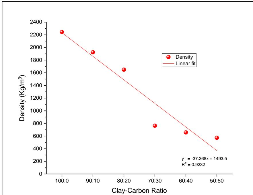
**Figure 1.** Relationship between the sample's density and the clay-carbon composition
