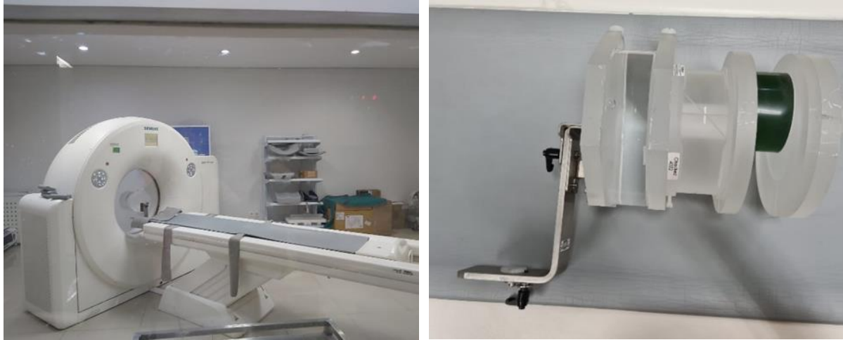
Figure 1. Siemens Somatom Scope CT-Scanner (left), and Siemens Water phantom (right)
