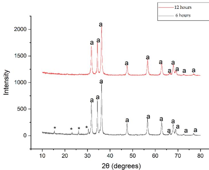
**Figure 2.** Results of XRD characterization of ZnO samples for holding times of 6 and 12 hours, (a) ZnO and (\*) Impurity.
