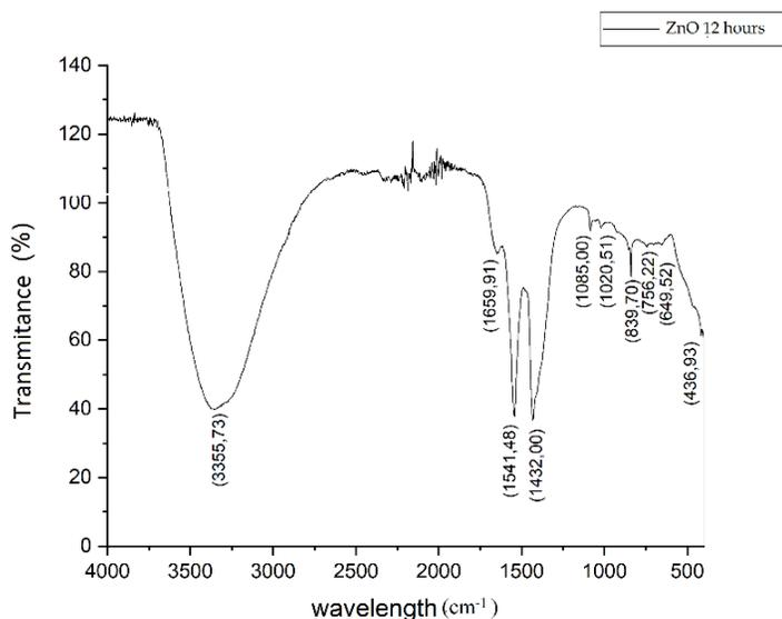
Figure 3. Results of FTIR characterization of ZnO samples
