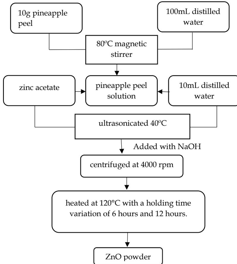
**Figure 1.** ZnO flow chart of pineapple peel extract
